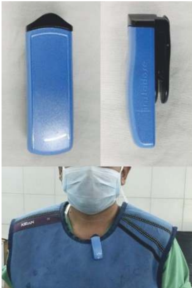
Figure 1: Image showing the The Instadose™ dosimeter and the method of wearing it during surgery
