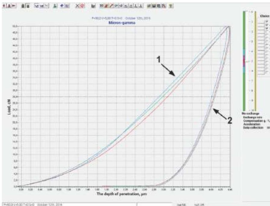
**Fig. 2: The Load Diagram of the Site of Implantation of Osteoplastic Material "ChronOS™" by Trihedral Diamond Pyramid of Berkovich on Indentometr "Micron-gamma". The Curve of Loading (1) and Unloading (2).**
