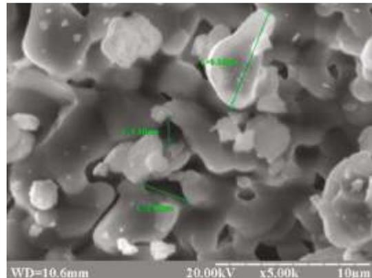
**Fig. 1: Microstructure of the Osteoplastic Material Calc-I-Oss®. Mineral Crystals Measuring 6.59 Microns and Micropores between them Ranging in Size from 1, 5 to 2, 89 Microns. Electronic Scanning Image X 5000**
